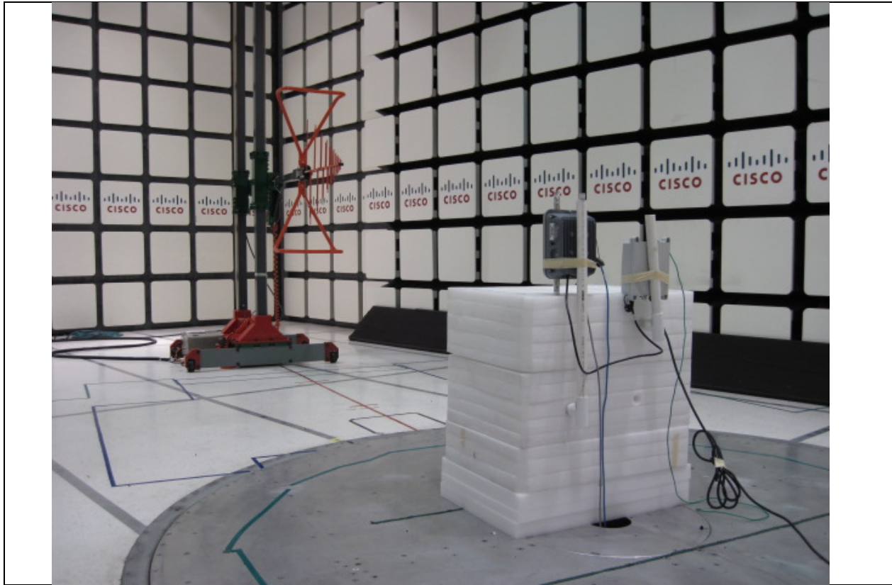
Title: Radiated Emissions 30-1000MHz Configuration Photograph
