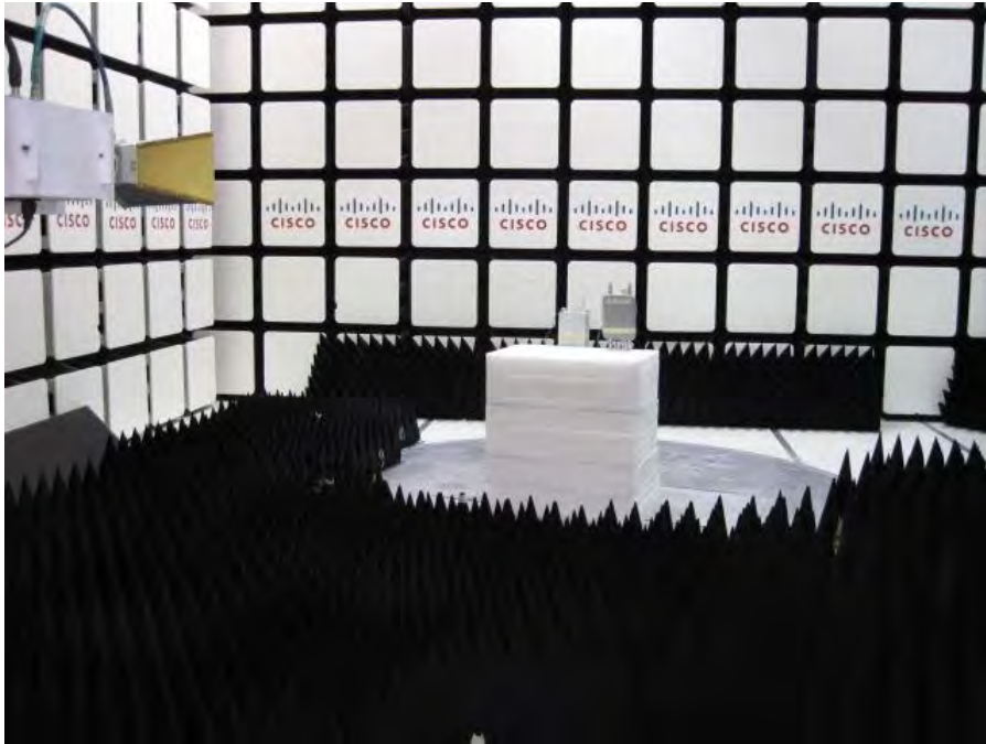
Radiated Test Setup 1–18GHz
