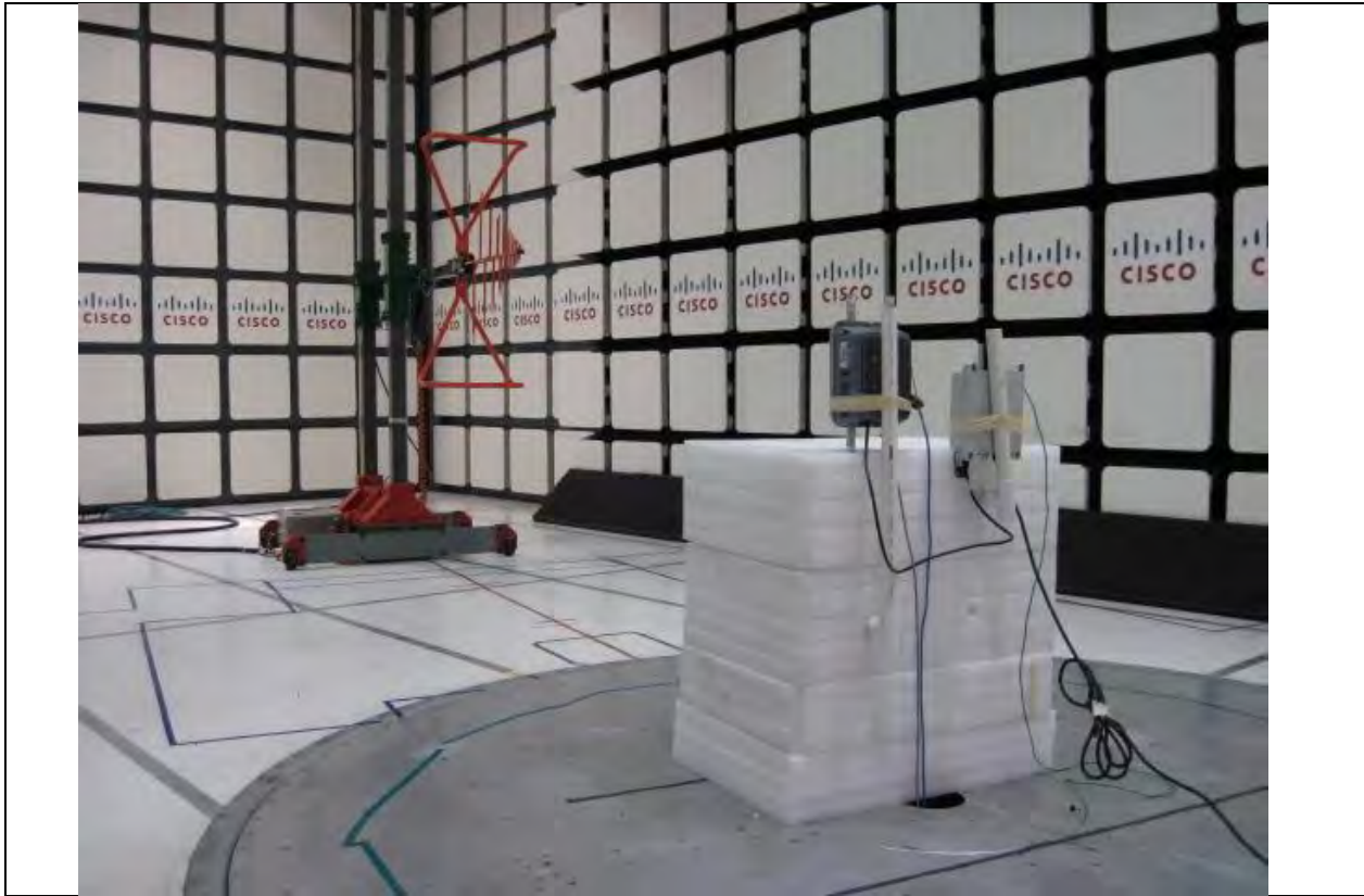
Title: Radiated Emissions 30-1000MHz Configuration Photograph
