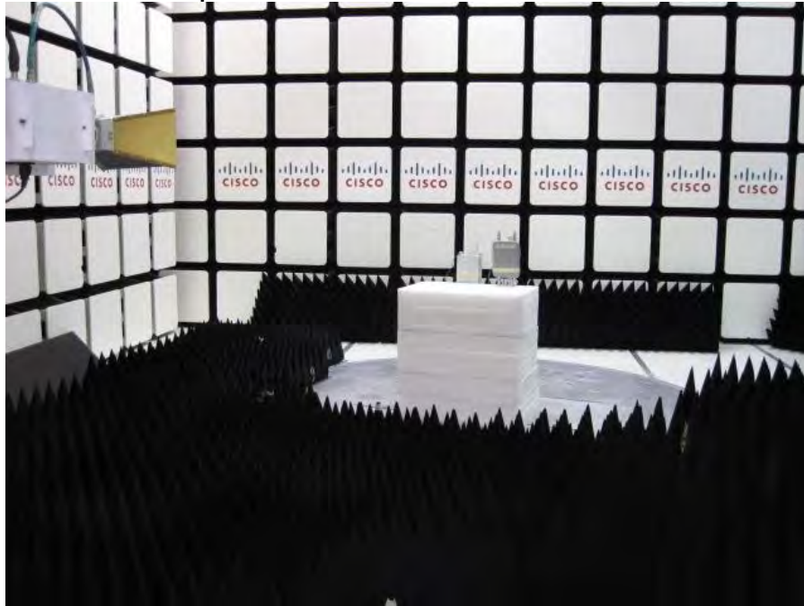
Radiated Test Setup 1–18GHz
