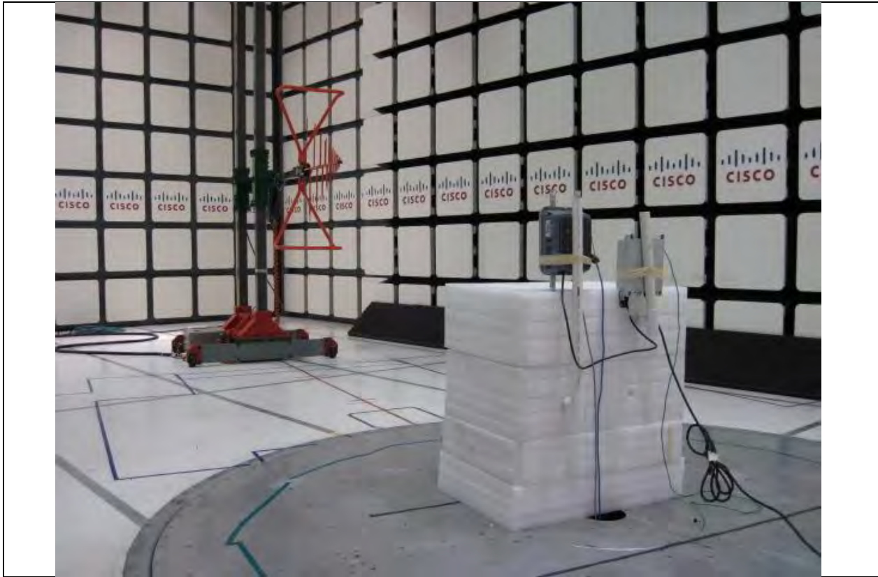
Title: EMC Radiated Emissions Configuration Photograph
