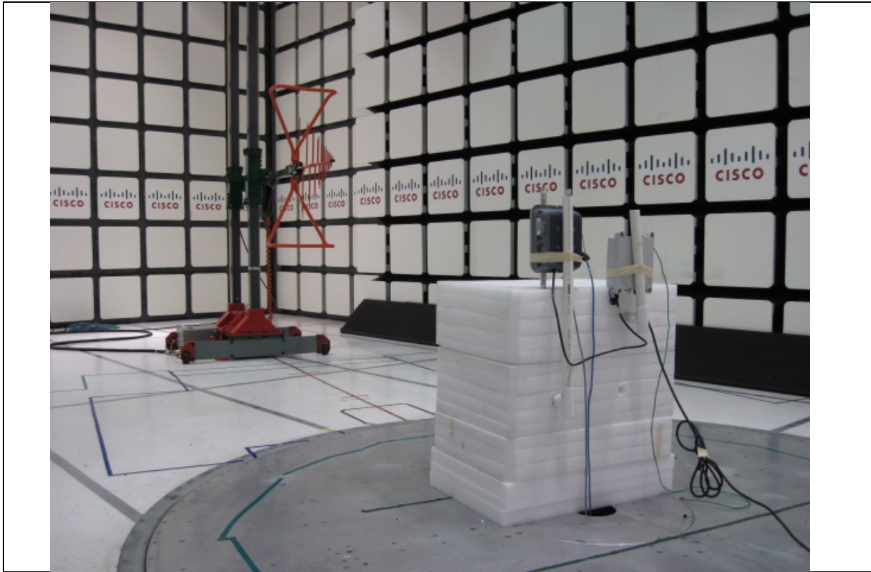
Title: Radiated Emissions 30-1000MHz Configuration Photograph
