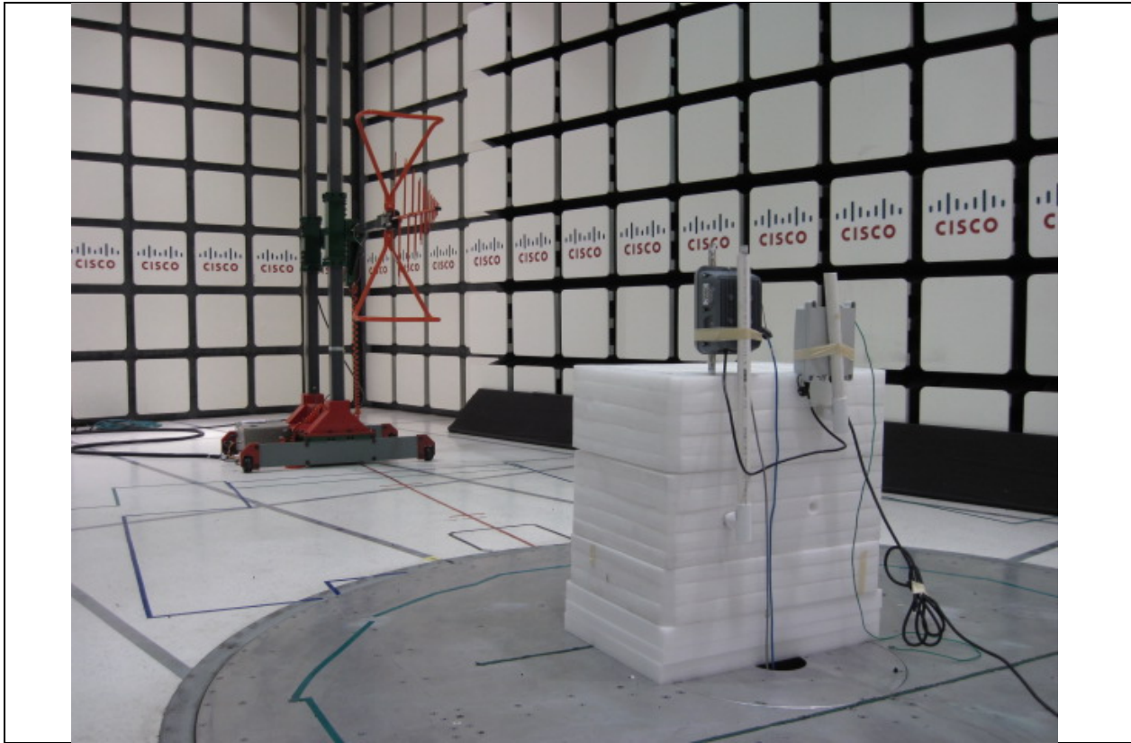
Title: EMC Radiated Emissions Configuration Photograph
