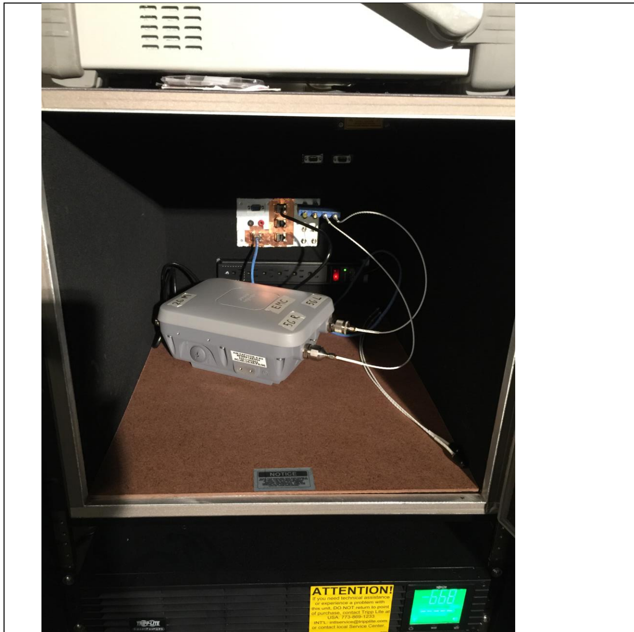
Title: AIR-CAP1532E-B-K9 Conducted Test Setup
