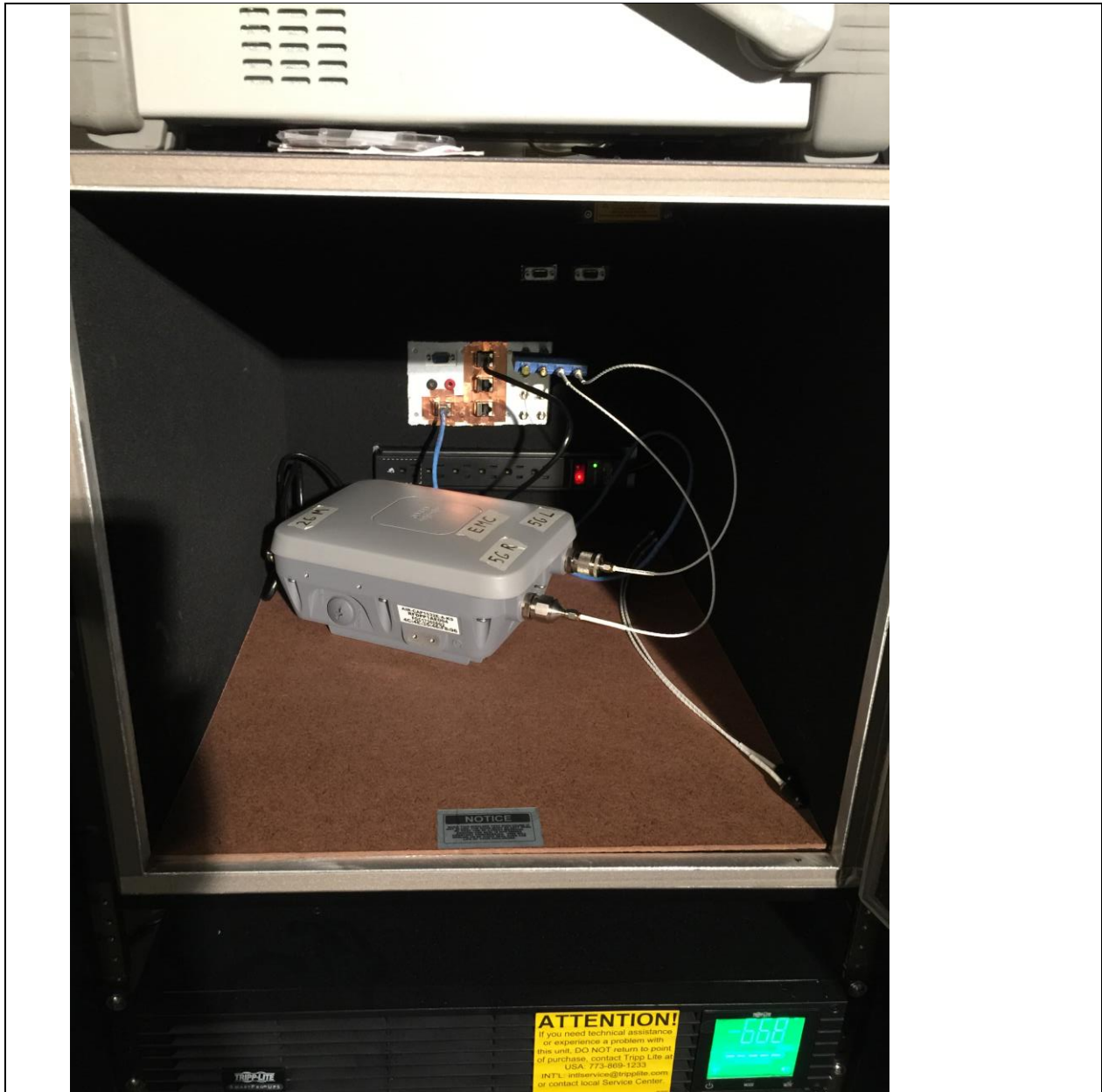
Title: AIR-CAP1532E-B-K9 Conducted Test Setup
