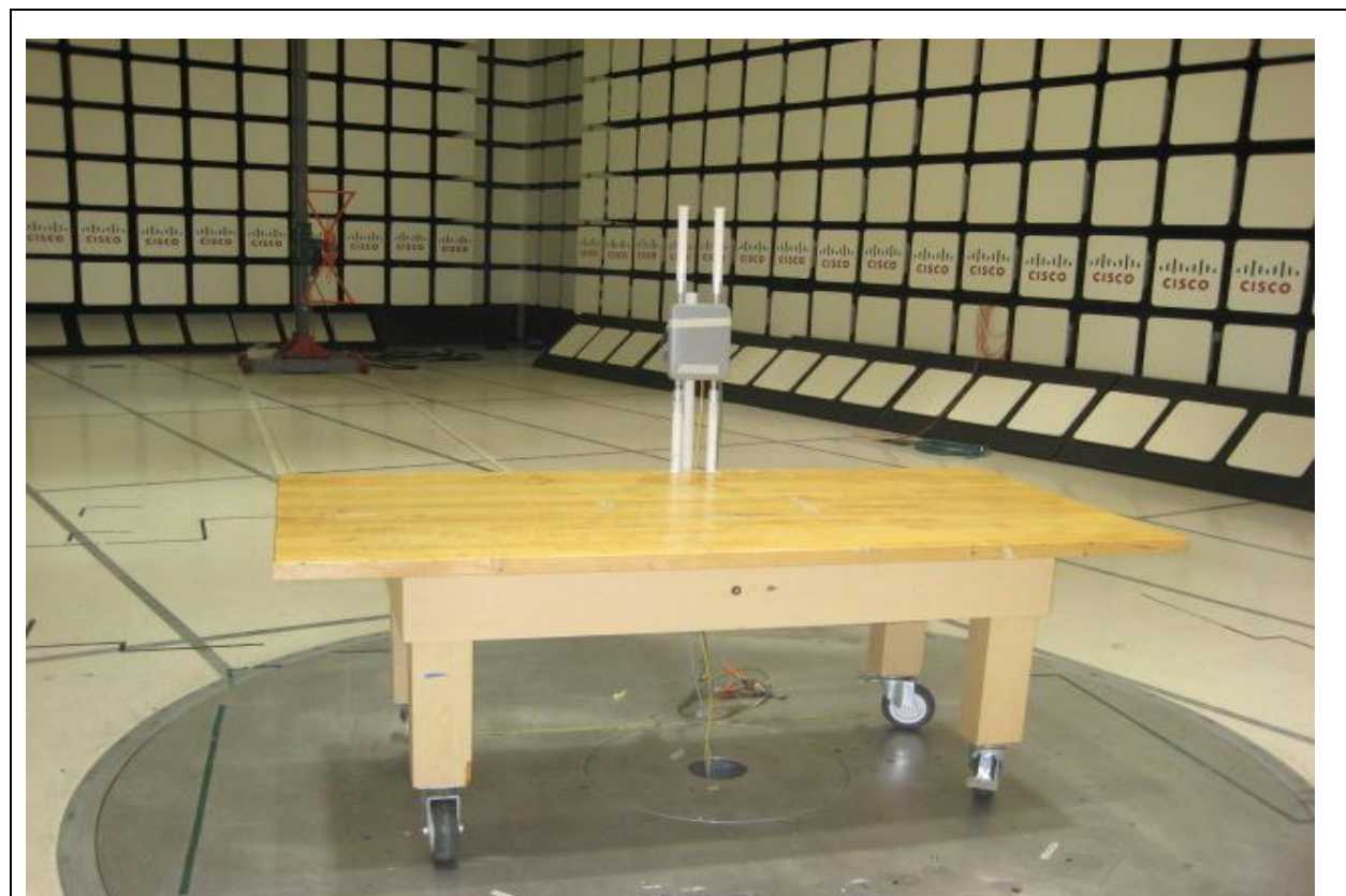
Title: Radiated Emissions 30-1000MHz Configuration Photograph
