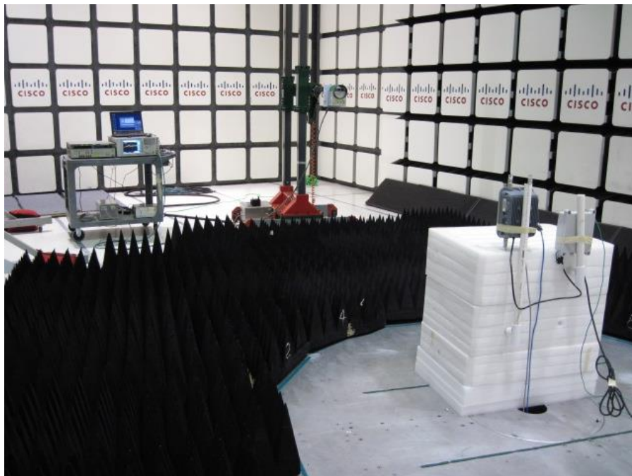
Radiated Test Setup 18-40GHz
