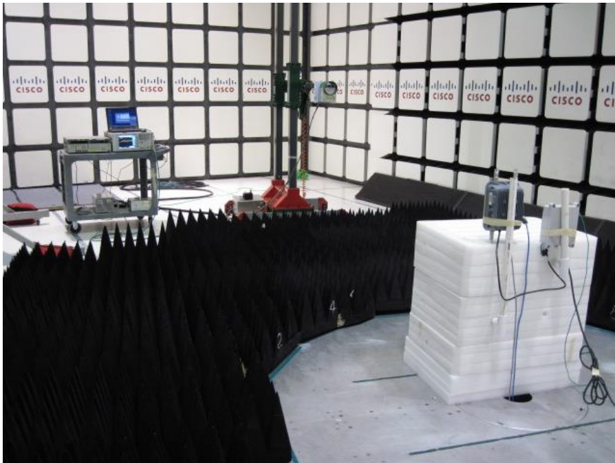
Radiated Test Setup 18–40GHz
