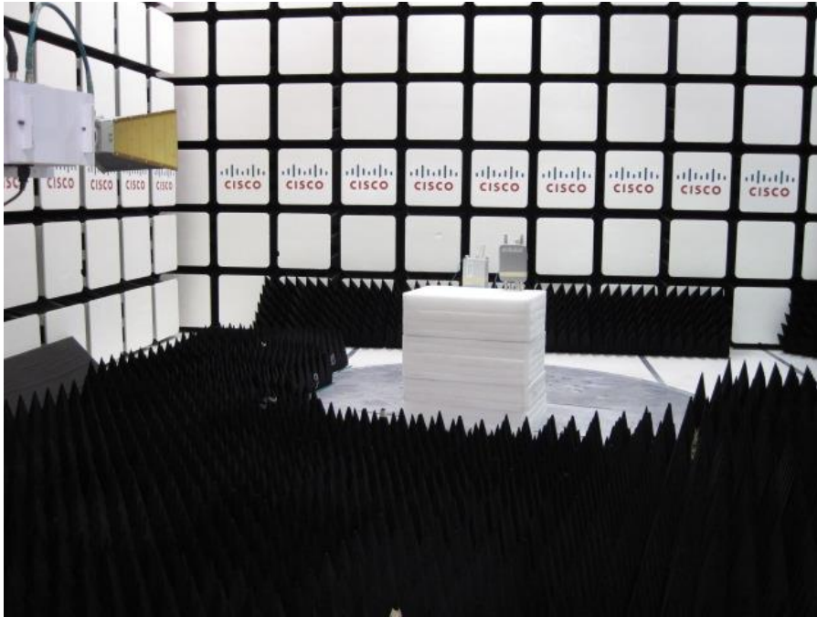
Radiated Test Setup 1–18GHz
