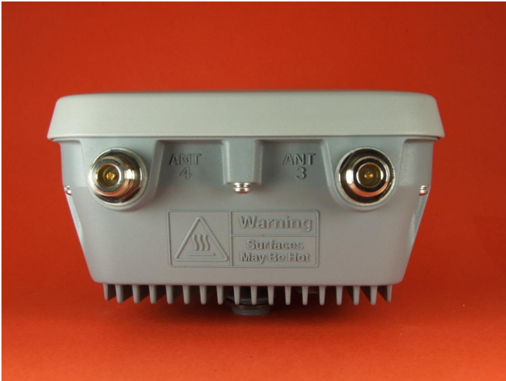
Top – Single band 5GHz ports
