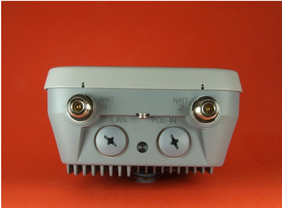
Bottom - Dual band/Single band 2.4GHz ports
