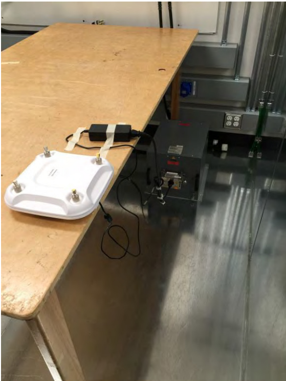
AIR-CAP3702P-B-K9 AC Conducted Emissions setup photo
