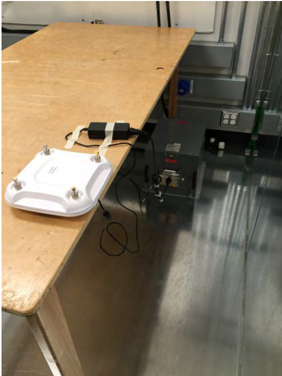
AIR-CAP3702P-B-K9 AC Conducted Emissions setup photo
