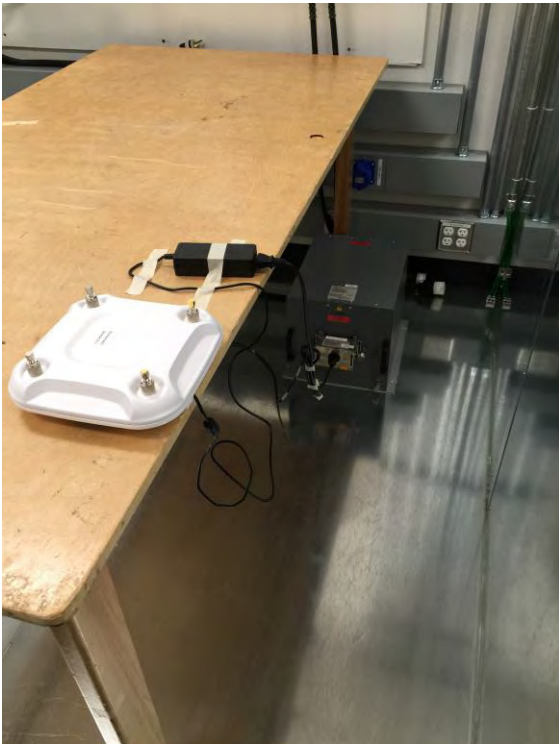
AIR-CAP3702P-B-K9 AC Conducted Emissions setup photo
