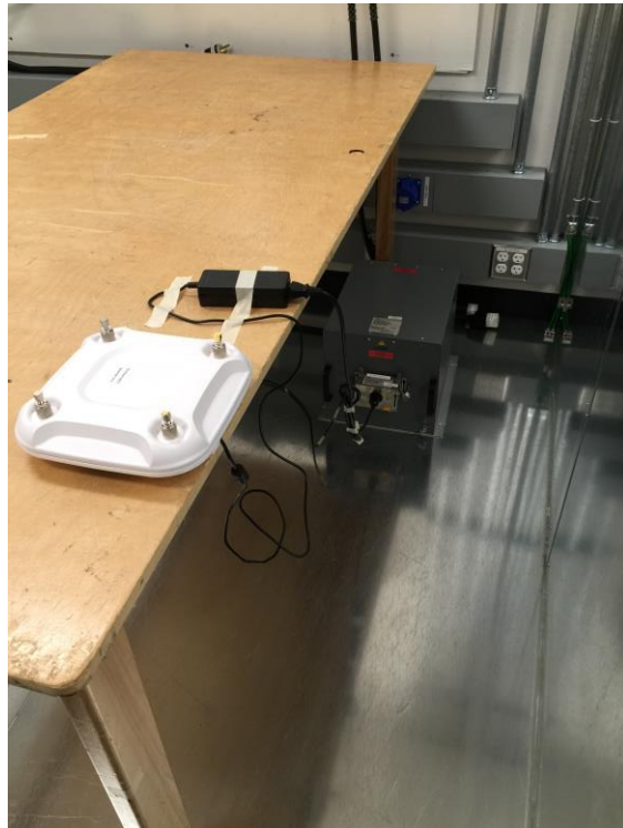
AIR-CAP3702P-B-K9 AC Conducted Emissions setup photo
