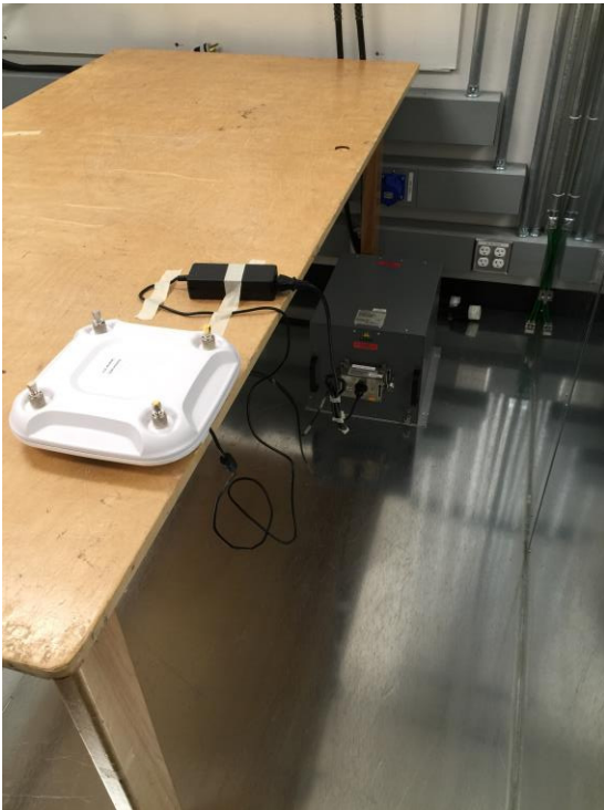
AIR-CAP3702P-B-K9 AC Conducted Emissions setup photo
