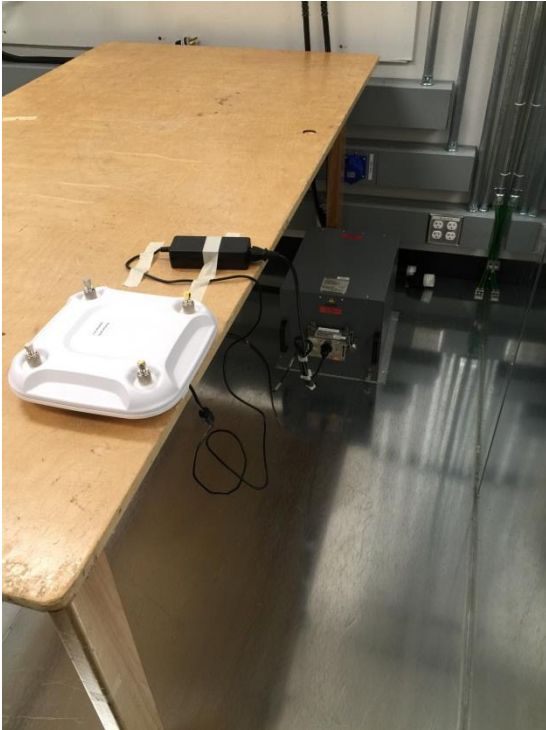
AIR-CAP3702P-B-K9 AC Conducted Emissions setup photo
