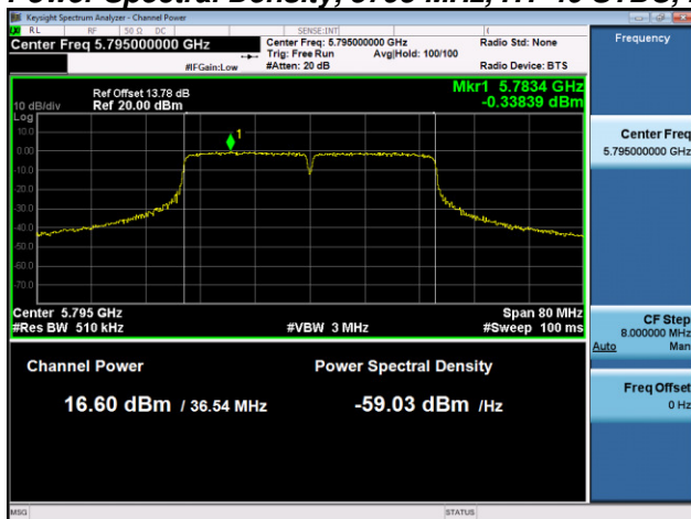
Power Spectral Density, 5825 MHz, Non HT-20, M0 to M15, M0 to M9 1-0ss
