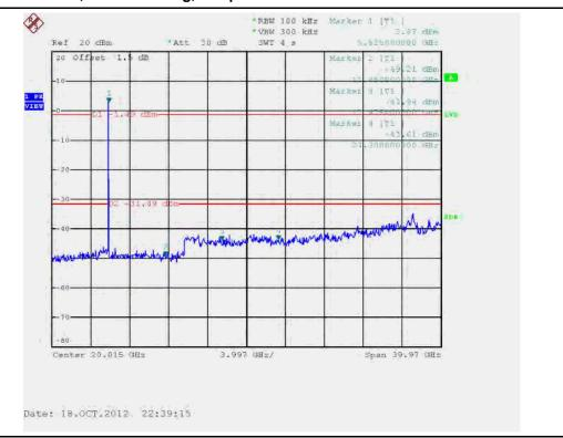
Transmitter Conducted Unwanted Emissions Plot on 5825 MHz, HT-20 / HT-20, STBC / HT-20, Beam Forming, M0
