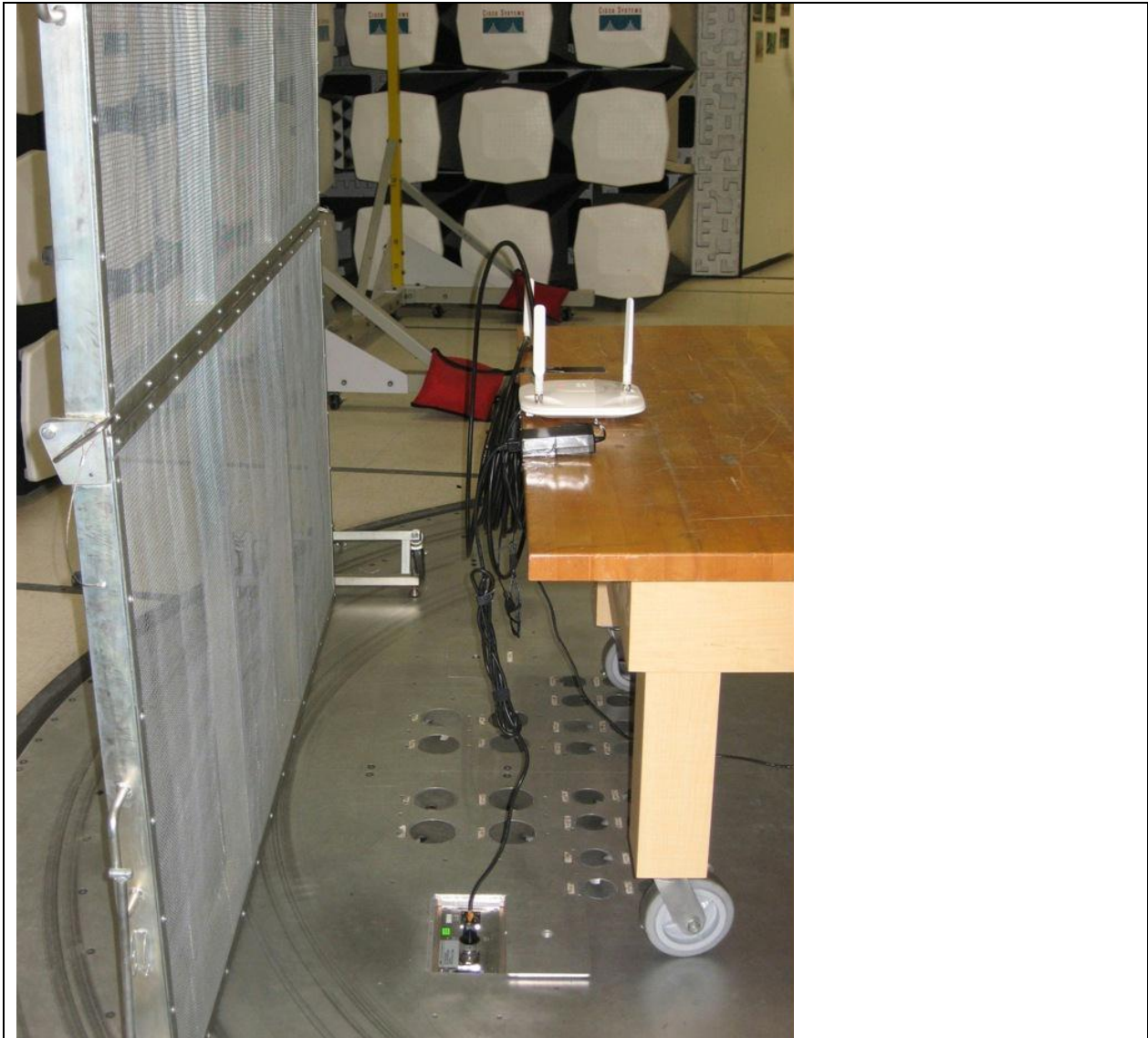
Conducted Emissions Configuration Photograph
