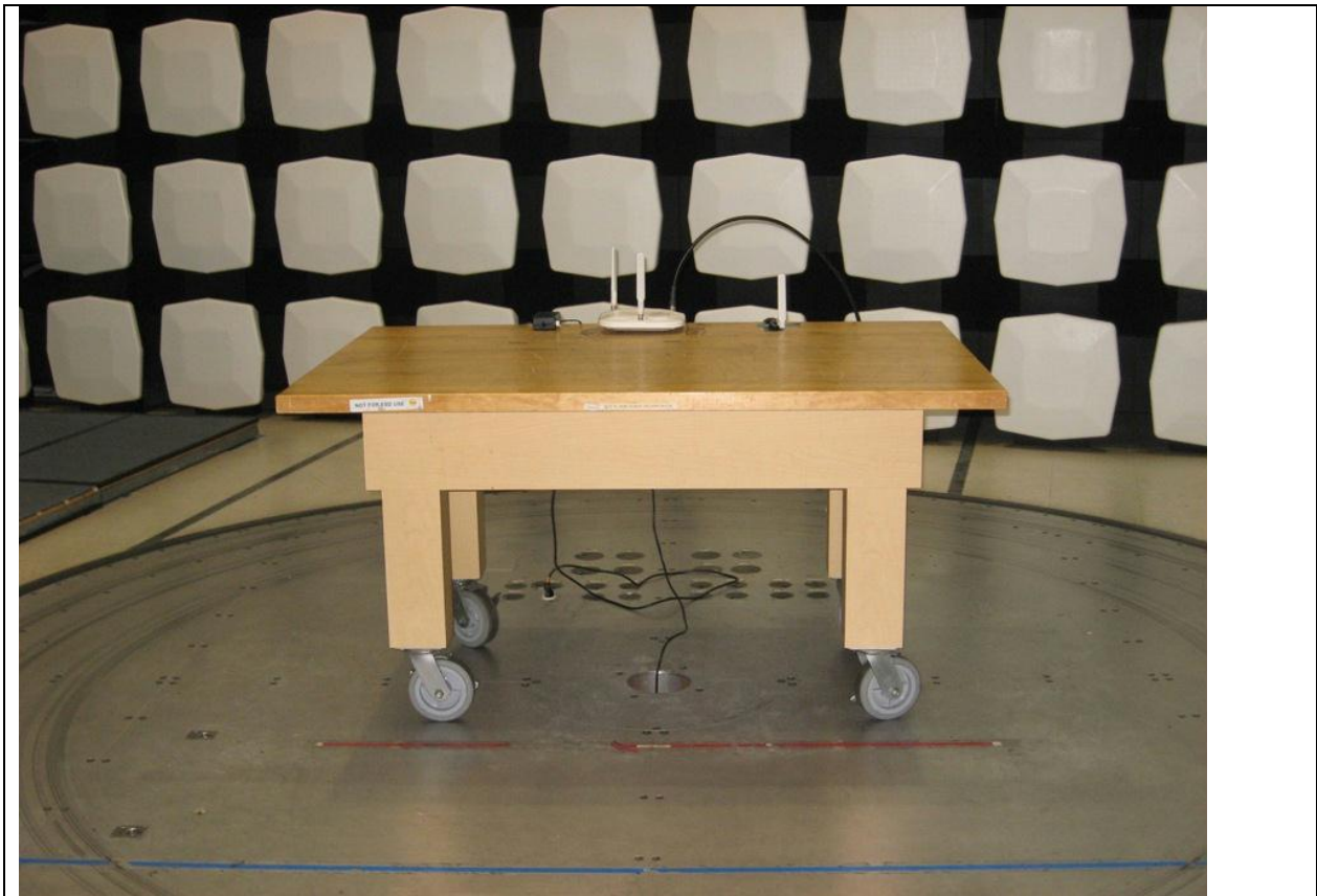
Radiated Emissions Configuration Photograph
