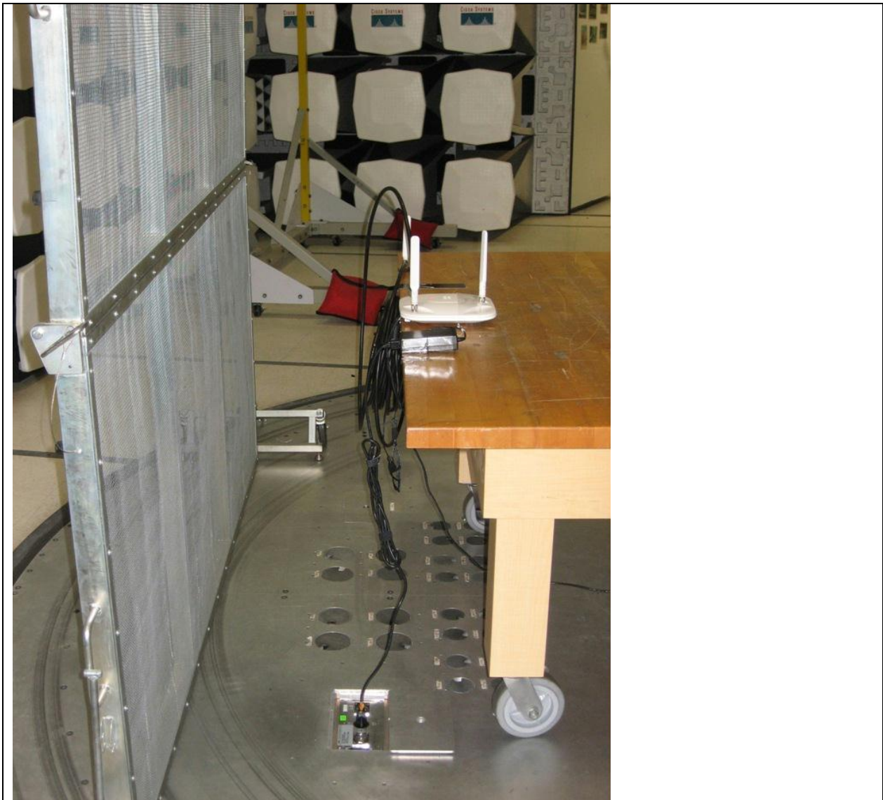
Conducted Emissions Configuration Photograph
