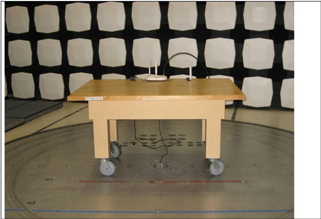
Radiated Emissions Configuration Photograph
