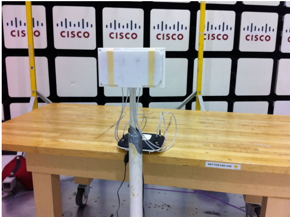
2.4/5 GHz Dual Band 6dBi MIMO patch antenna
