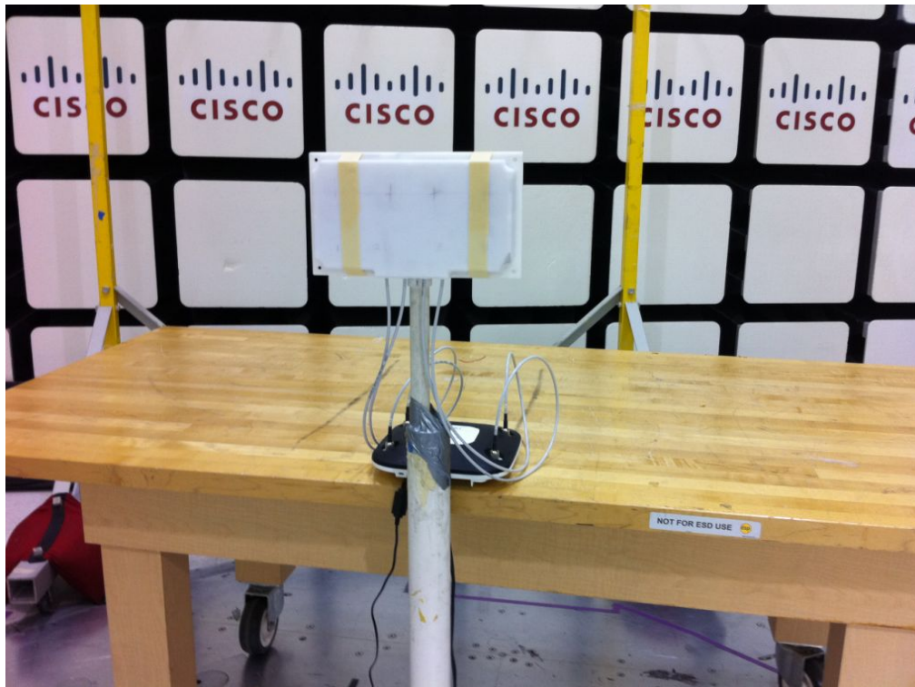
5GHz 6dBi MIMO Patch Antenna co-Located with 2.4GHz 6dBi MIMO Patch Antenna
