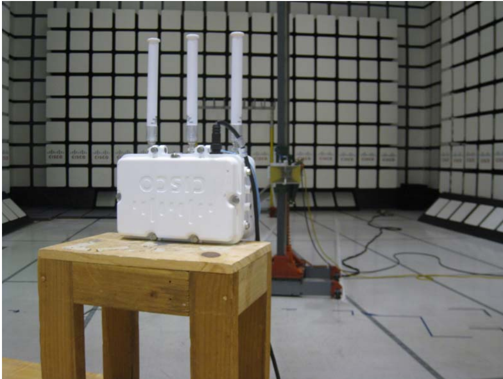
External 2.4/5GHz antenna (4/7 dBi)
