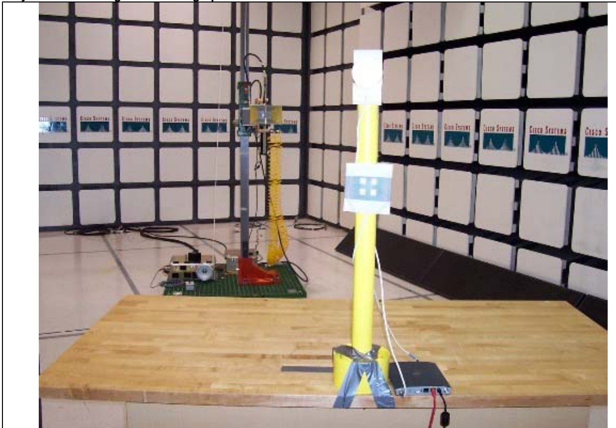
Title: Colocation Tests with 2.4GHz 10dBi Yagin and 5GHz 9.5dBi Patch Antennas
