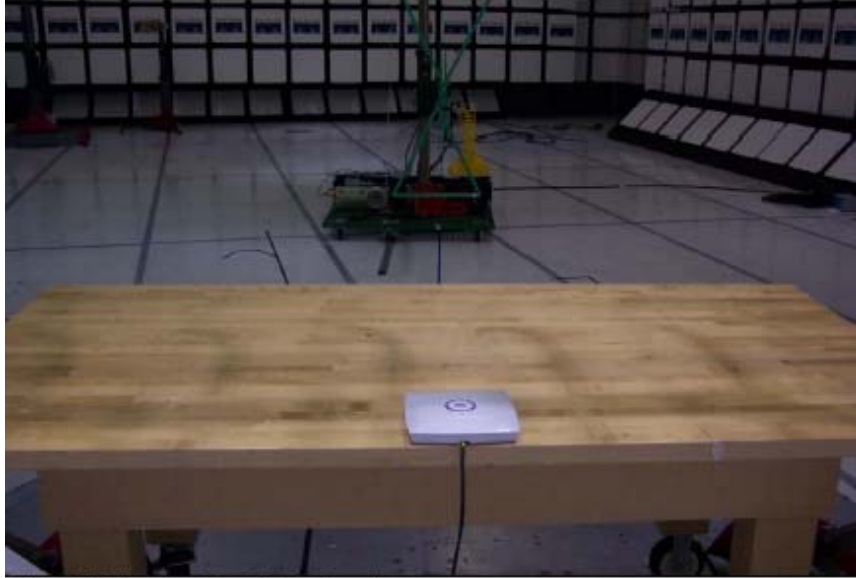
Title: 3m Radiated Emissions Test Configuration
