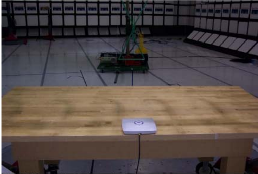
Title: 3m Radiated Emissions Test Configuration
