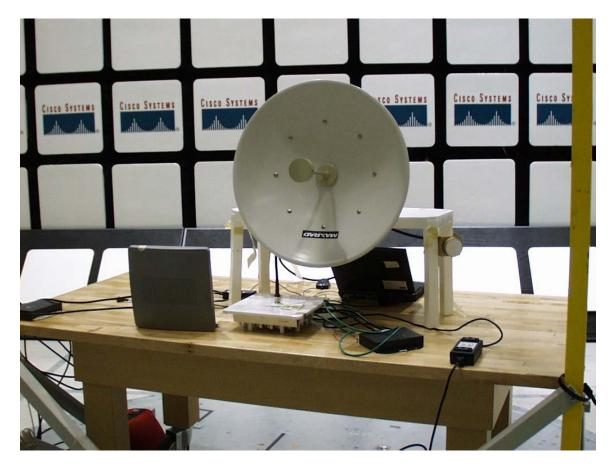
Radiated Emissions testing  $1-40~\mathrm{GHz}$
