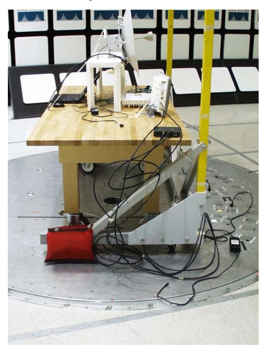
Radiated Emissions testing  $1-40~\mathrm{GHz}$
