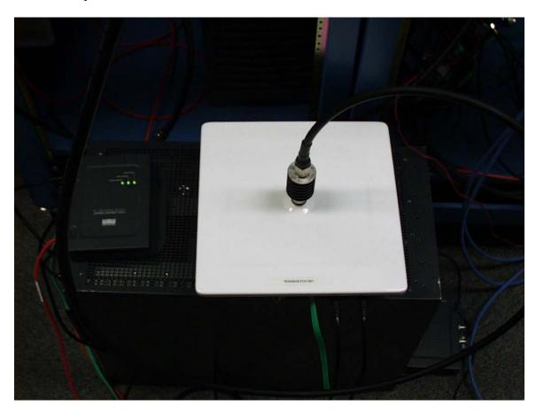
Radiated Emissions Test Set-up, 30 – 1000 MHz
