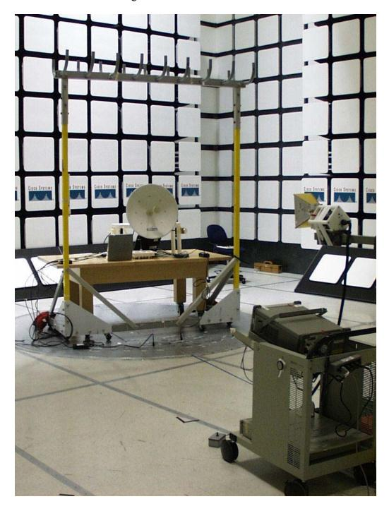
Radiated Emissions testing 1 – 40 GHz
