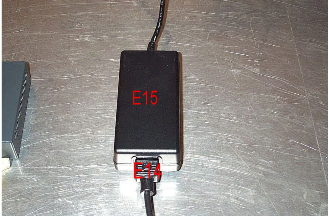
ESD Test Points: Spier power supply
