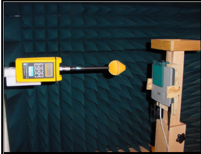
PHOTOGRAPH 3.2.2: WALL-MOUNTED EUT WITH THE 2.2 DBI DIPOLE ANTENNAS; ALL ANT ENNAS ARE IN THE HORIZONTAL POSITION
