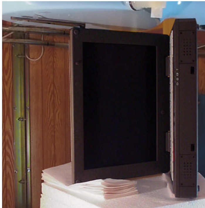
SAR measurement setup with the antenna at 0.25cm from the phantom surface.
