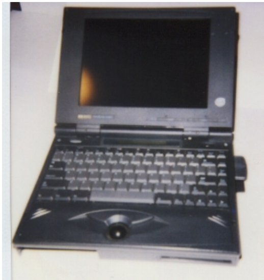
Fig. 1. Photograph of Cisco/Aironet Model LDK102040 Wireless PC with RF antenna inserted at the back on the right-hand side of the keyboard.
