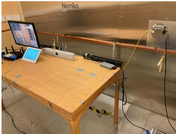
Power-Line Conducted Emissions
