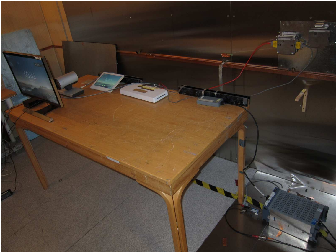
Power line Conducted Emissions Test
