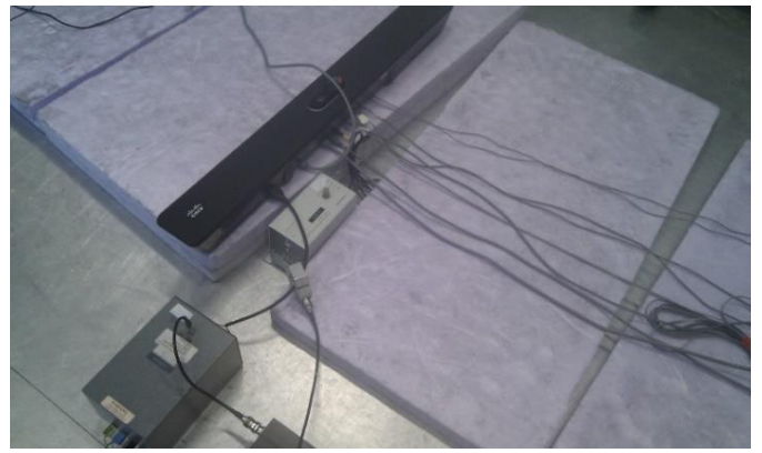
Test set-up for Conducted RF disturbance immunity (AC mains)
