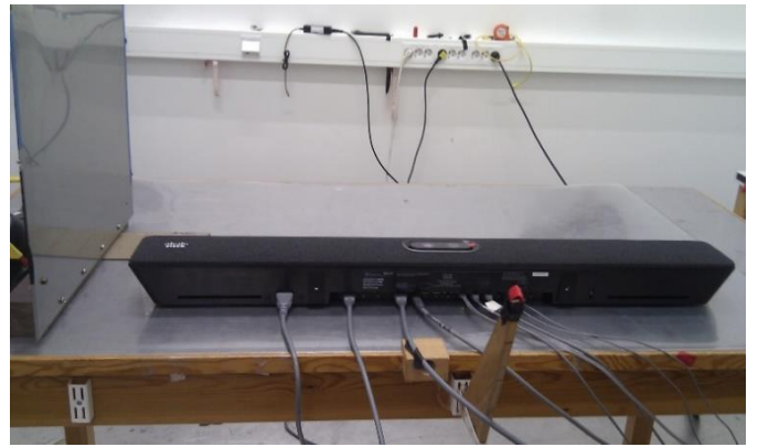
Test set-up for Electrostatic Discharge (ESD) Immunity
