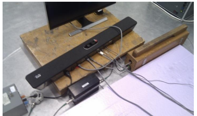
Test set-up for Conducted RF disturbance immunity (Signal ports)
