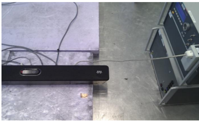
Test set-up for Electric fast transients, Surge and Voltage dips and interruptions immunity (AC mains)
