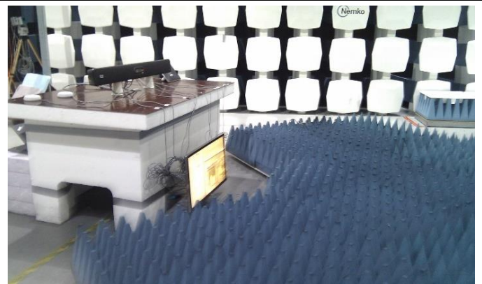
Test set-up for Radiated emissions measurements (6-12 GHz, FCC)
