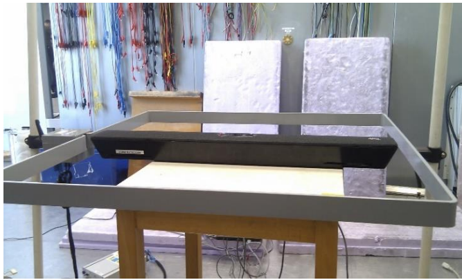
Test set-up for Power Frequency Magnetic Field Immunity.
