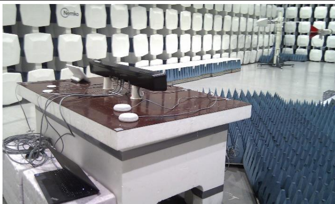
Test set-up for Radiated emissions measurements (6-12GHz, FCC)
