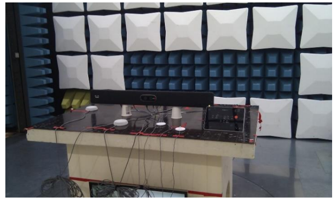
Test set-up for Radiated emissions measurements (1-6 GHz, FCC)
