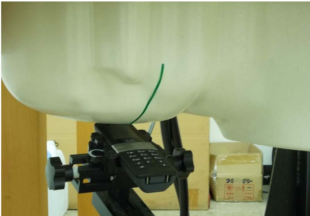
Measurement Position of Right-Tilt (RT) with Handset
