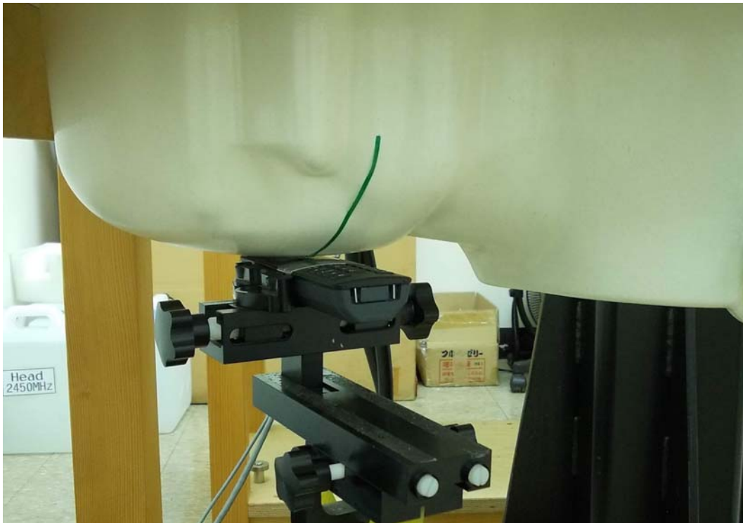
Measurement Position of Right-Cheek (RC) with Handset
