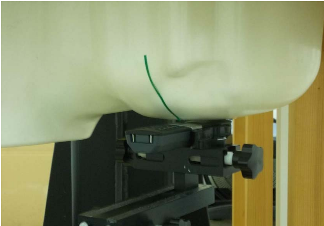
Measurement Position of Left-Cheek (LC) with Handset
