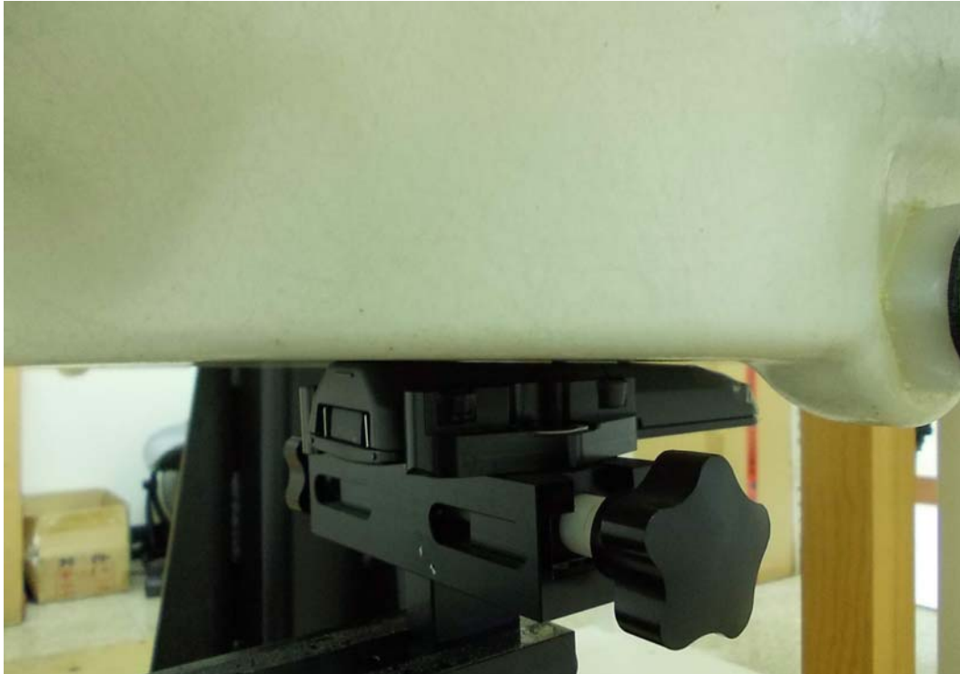
Measurement Position of Body Rear-UP with Handset
