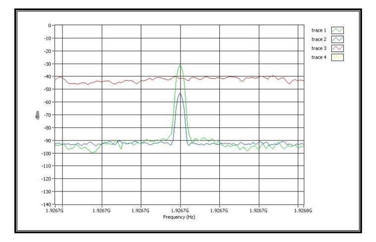
Comment1: Trace1 (green) is the interference on all 5 carriers. The level is Tu+UM+10dB. Comment2: Trace2 (blue) is interference on all 5 carriers. The level is TuR. Comment3: Trace3 (Red) is the EUT begins to transmit the beacon when interference level is TuR. Comment: 7.3.3b
