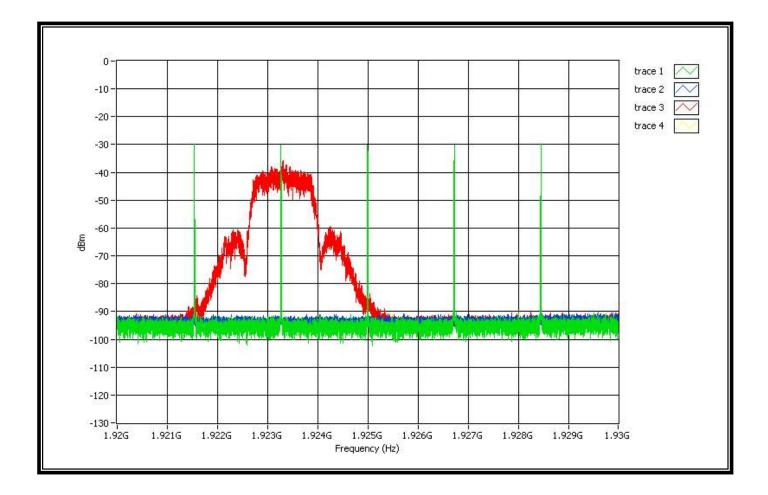
Comment1: Trace1 (green) is the interference on all 5 carriers. The level is Tu+UM+10dB. Comment2: Trace2 (blue) is interference on all 5 carriers. The level is TuR. Comment3: Trace3 (Red) is the EUT begins to transmit the beacon when interference is TuR.
