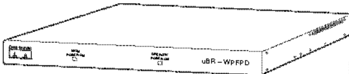
Figure 5 Power Feed Panel (Front Panel)
