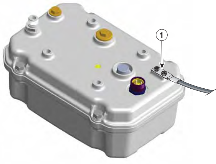
Figure 2-18 Installing the Ground Lug
