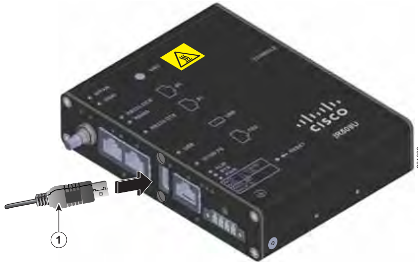
Figure 2-27 Connecting the USB Cable Connector to the USB Port
