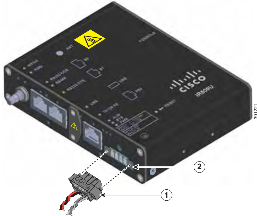
Figure 2-13 Removing the Power and Alarm Connector from the WPAN Gateway
