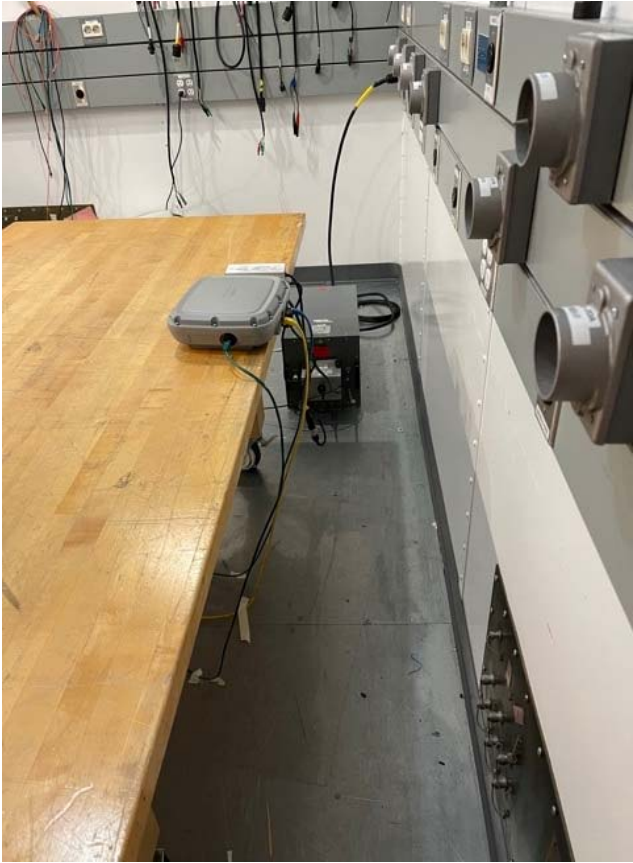
Title: AC Conducted Emissions Test Setup
