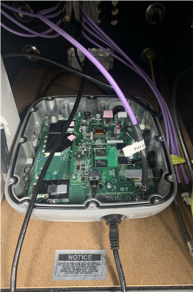
Title: Radio Conducted Test Setup – Rack 8 - BLE
