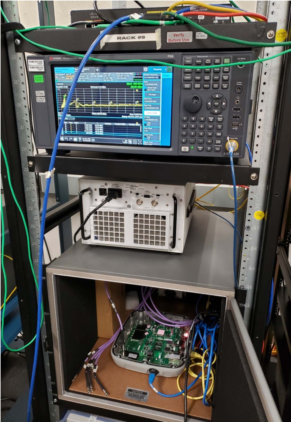
Title: Radio Conducted Test Setup – Rack 9
