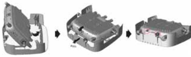
Figure 74: Installing the AP Cover Kit
