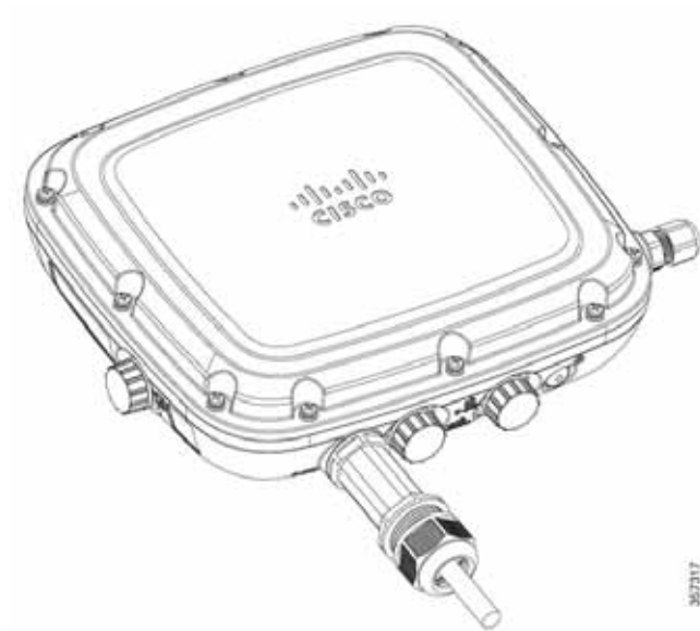
Figure 82: Fiber-Optic cable and gland installed to AP
