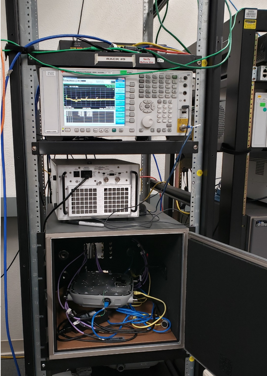
Title: Radio Conducted Test Setup – Rack 9 – BLE
