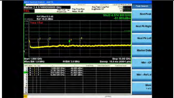
Mod: OFDM, Mode 144, 926.8MHz (1-10GHz) Peak
