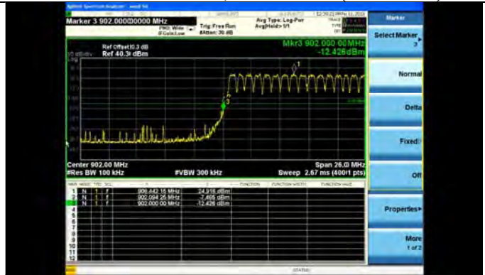
Modulation: OFDM, Mode: 146 (Lower BE)
