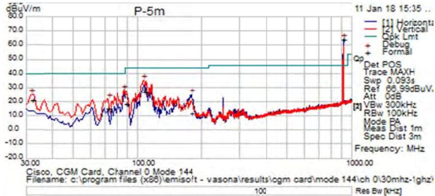
Title: TX Spurious Emissions from 30MHz-1GHz – Ch15(914.8 MHz)
