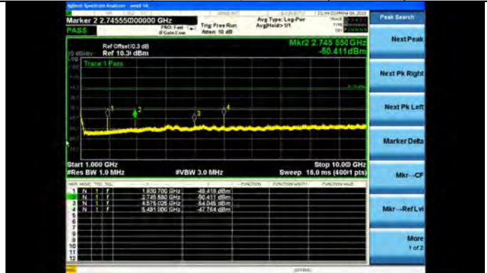
Mod: OQPSK, Mode 192, 927.8MHz (1-10GHz) Peak
