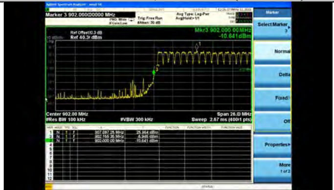
Modulation: OFDM, Mode: 146 (Lower BE)
