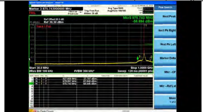
Mod: OQPSK, Mode 192, 927.8MHz (30-1GHz) Average
