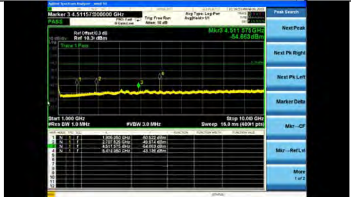
Mod: OQPSK, Mode 192, 915MHz (1-10GHz) Peak
