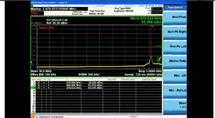
Mod: OQPSK, Mode 192, 927.8MHz (30-1GHz) Average
