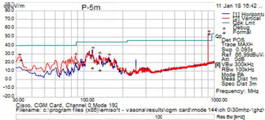
Title: TX Spurious Emissions from 30MHz-1GHz – Ch0 (902.2 MHz)
