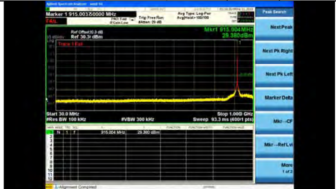
Mod: OQPSK, Mode 192, 927.8MHz (30-1GHz) Peak
