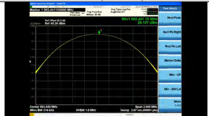
Modulation : 2FSK , Mode:98 , 915.2MHz
