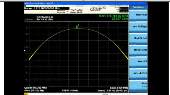
Modulation : 2FSK , Mode:98 , 927.6MHz
