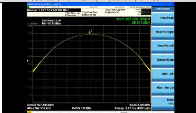
Modulation : 2FSK , Mode:66 , 927.6MHz
