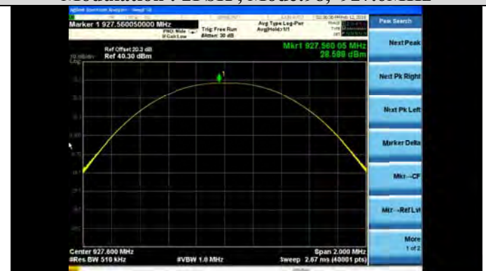
Modulation : 2FSK , Mode:98 , 927.6MHz
