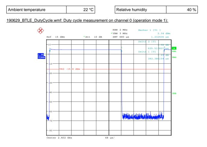
$$T_{TX_{On}} = 392.386 \,\mu_{S}_{\text{Date: }22.\text{AUG. }2019} \quad T_{TY_{S}CY_{S}cle} = 625.513 \,\mu_{S} \tag{1}$$
