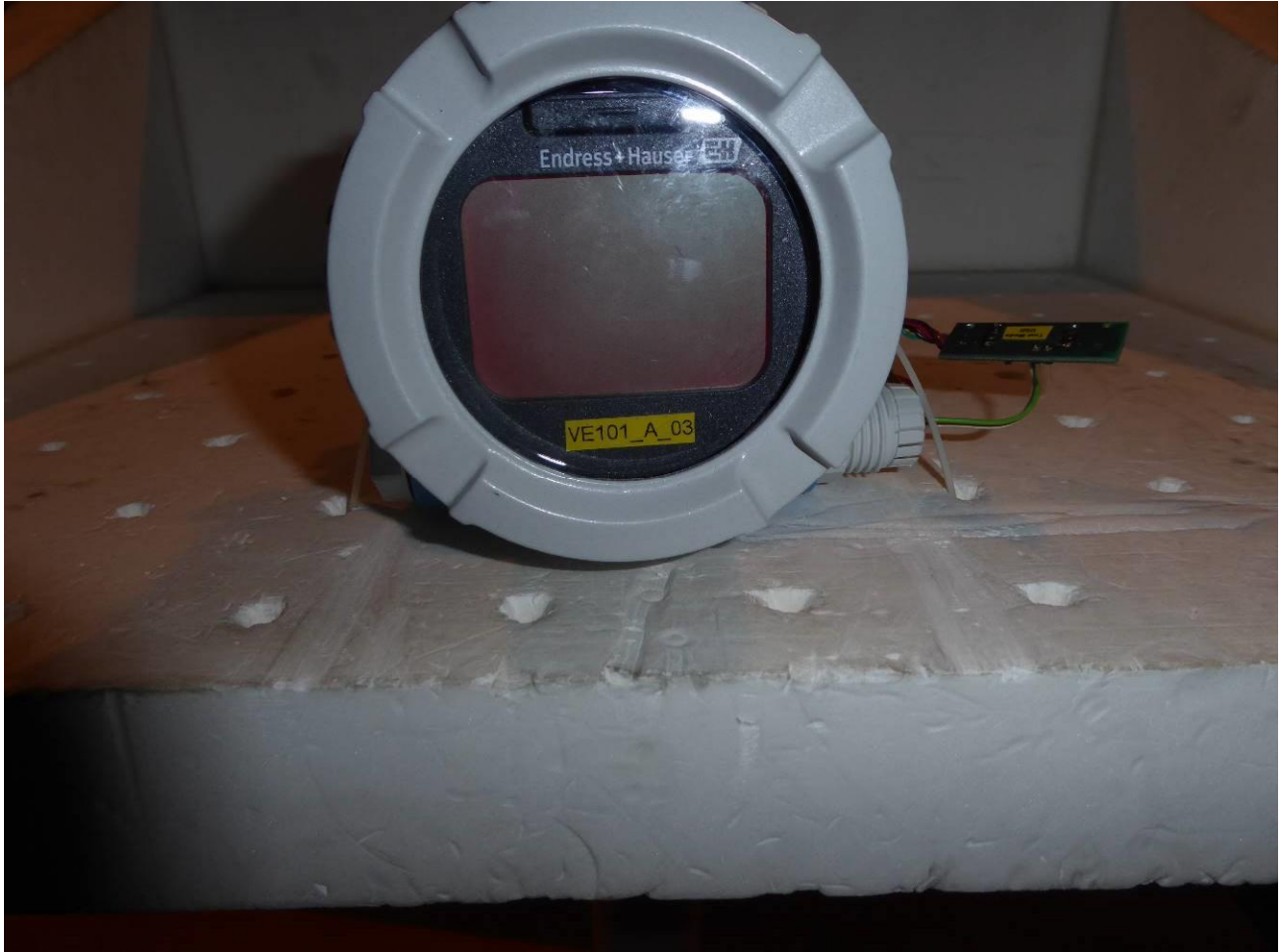
Test setup – radiated test in anechoic chamber
