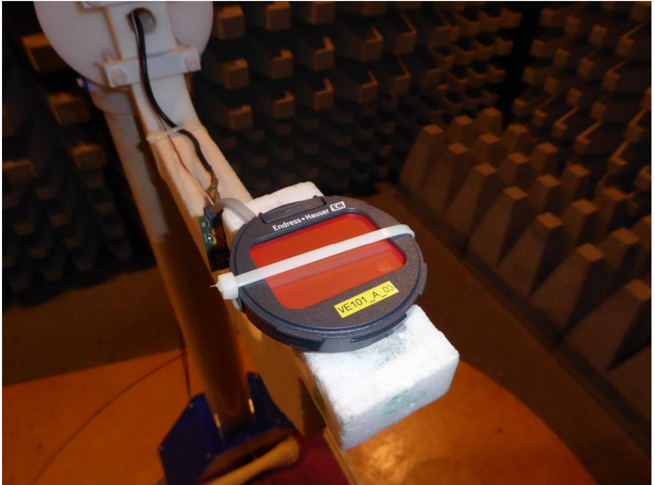
Test setup – radiated test in anechoic chamber
