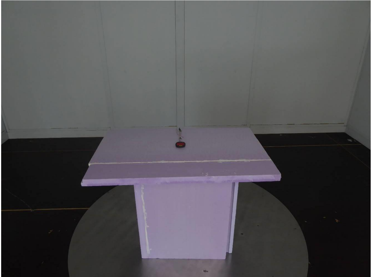
Test setup – radiated test on open area test site
