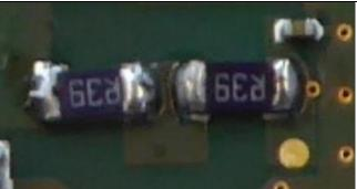
Replaced Ex Resistors (100 ohms + 47.8 ohms) with 0.39 ohms resistors to allow the high current draw of constant carrier mode
