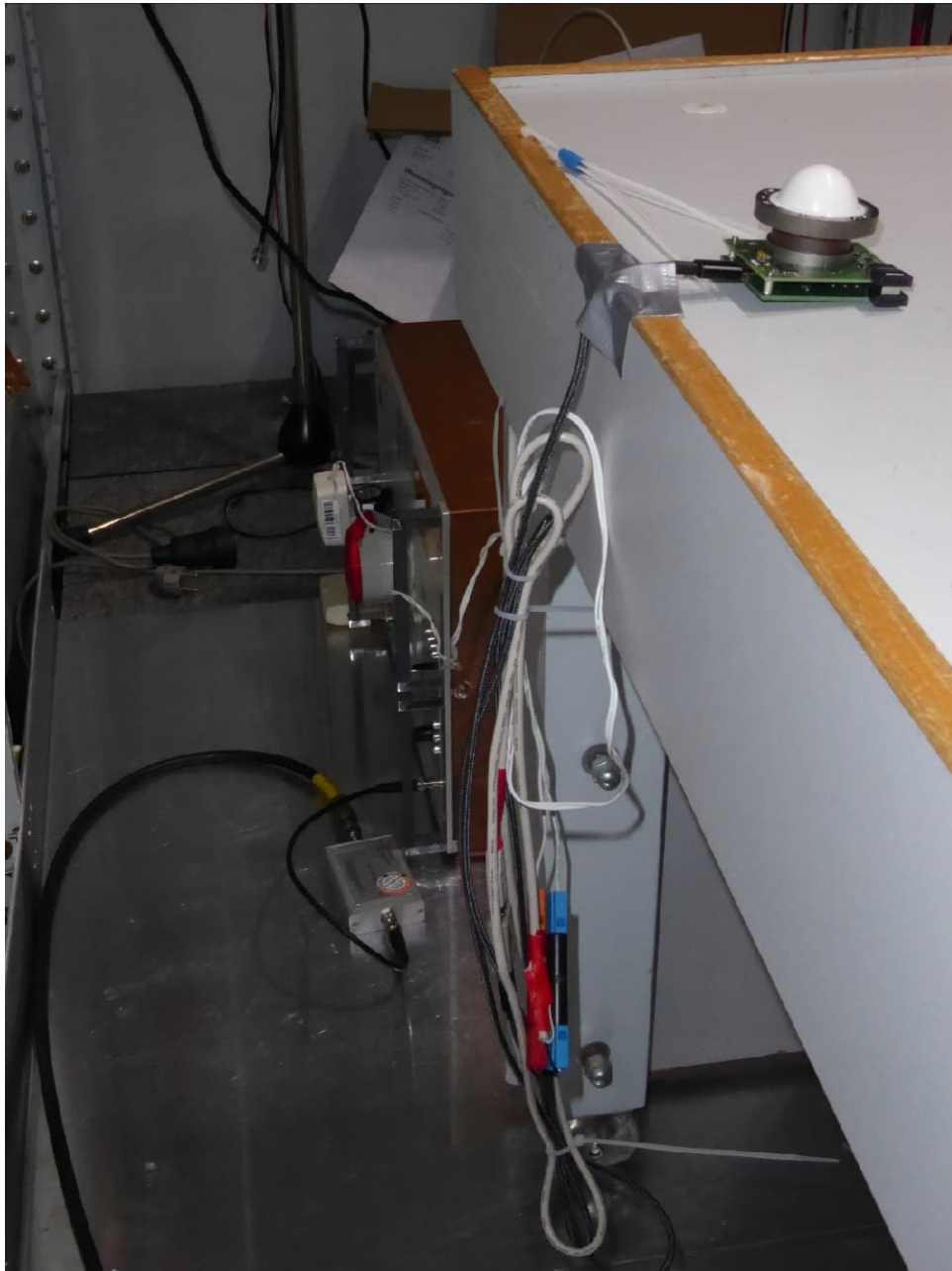
Test AC power line conducted emissions
