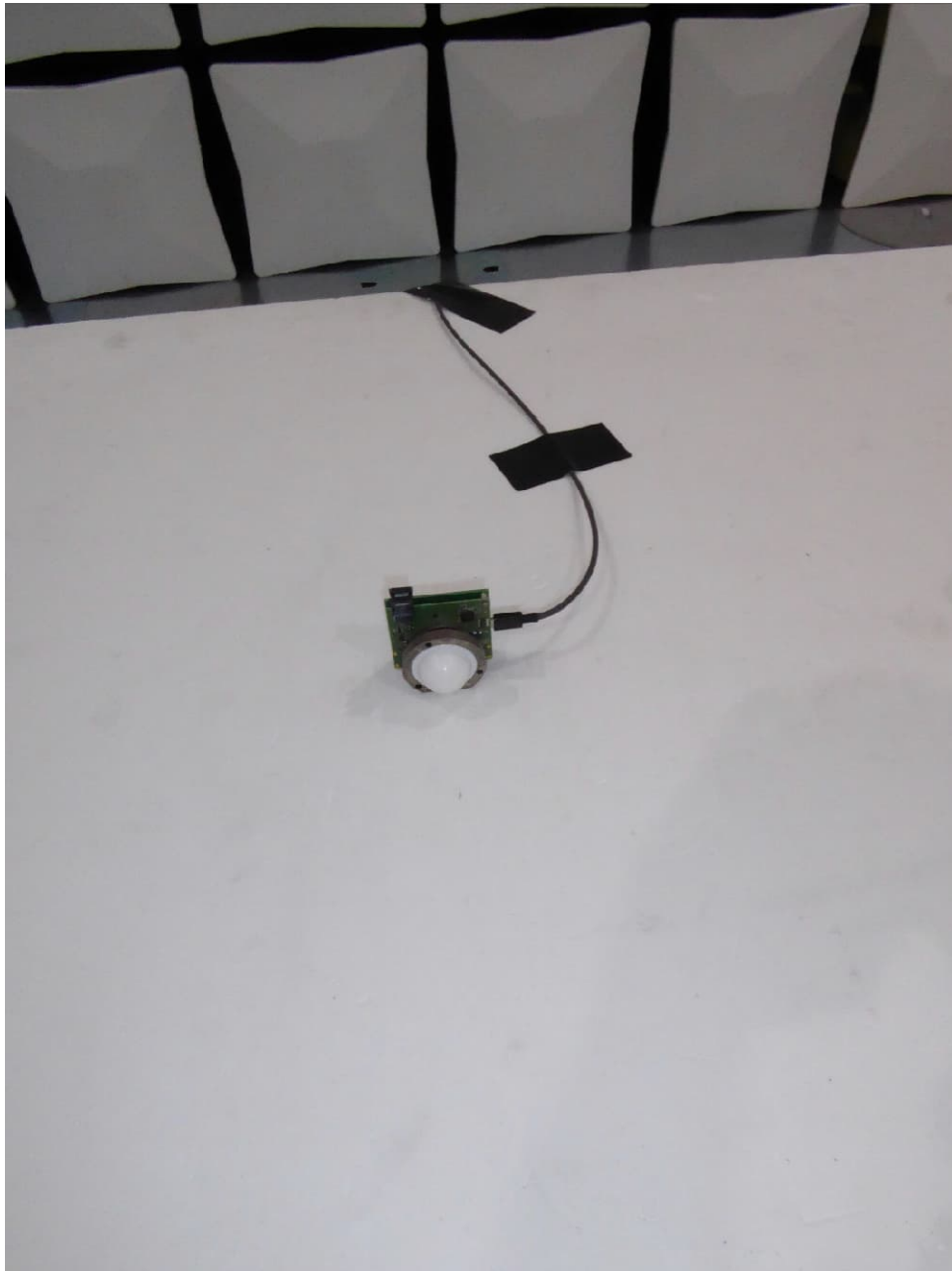
Test setup semi anechoic chamber (position 1)
