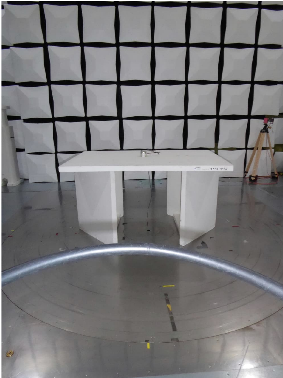
Test setup semi anechoic chamber (<30 MHz, position 1)
