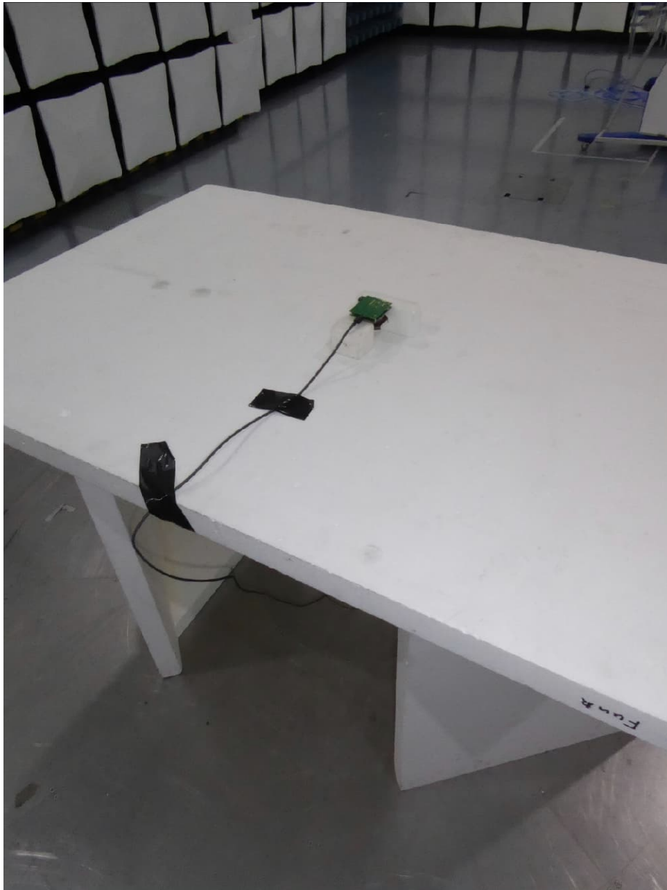
Test setup semi anechoic chamber (position 2)
