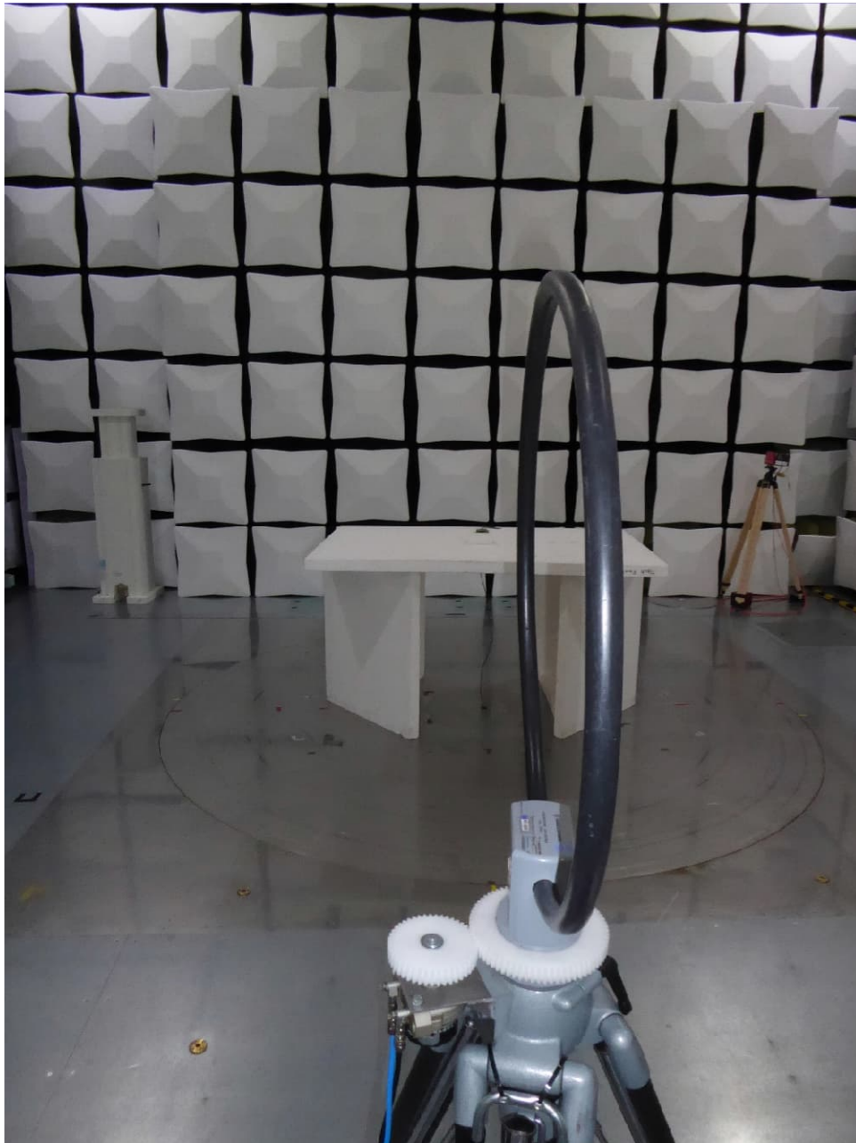
Test setup semi anechoic chamber (<30 MHz, position 2)
