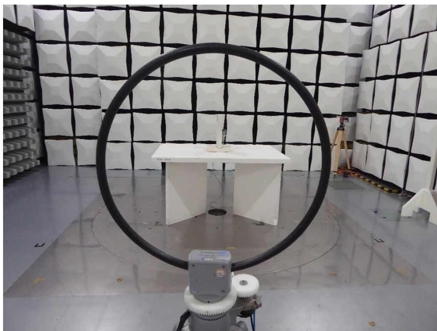
Test setup semi-anechoic chamber M276 Preliminary measurement
