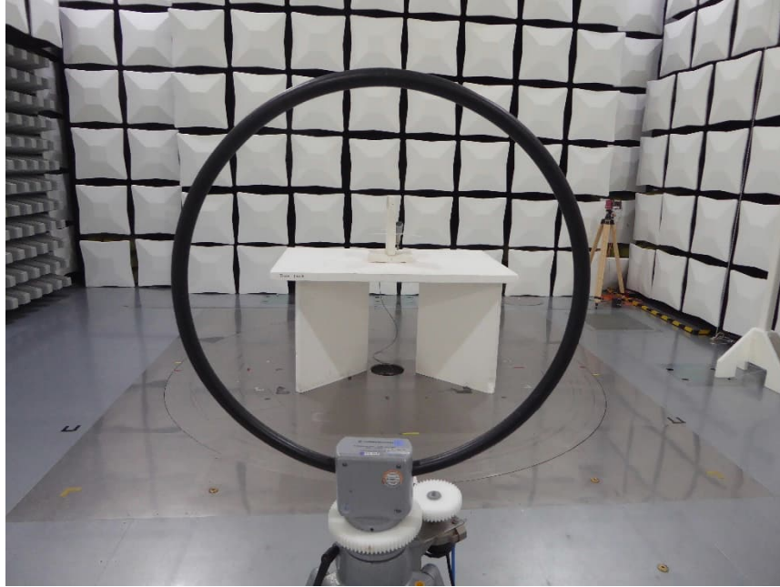
Test setup semi-anechoic chamber M276 Preliminary measurement
